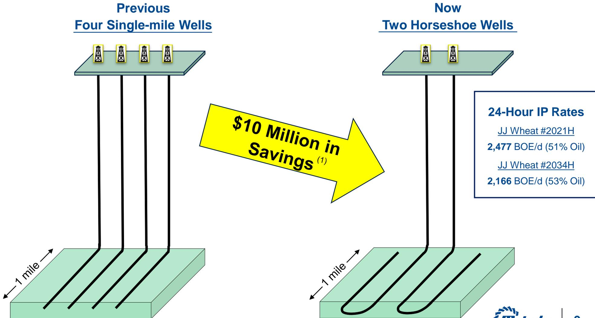
(1) Savings based on cost estimates for drilling four single-mile laterals versus two horizontal horseshoe well designs.
